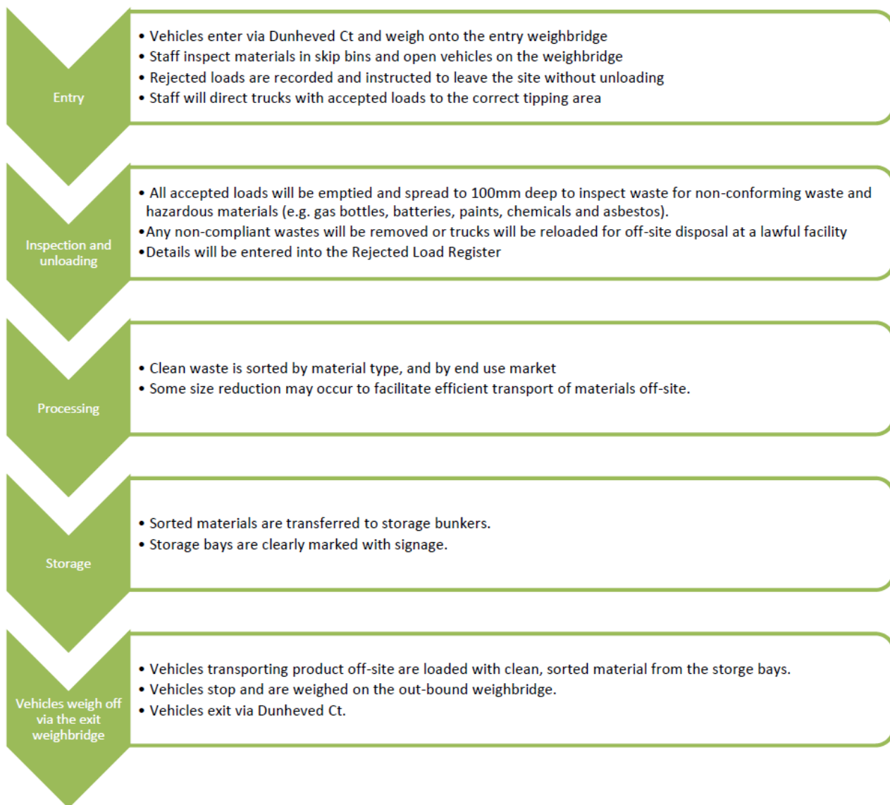
Figure 3. Process flow chart for the operation of the Waste Management and Recycling Facility.
